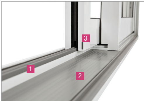
The saddle-rail sash design provides exceptionally smooth operation. Utilizing precision bearing rollers, the operation of the sash requires little effort and provides long-lasting, trouble-free operation. The attractive anodized sill tread complements the aesthetics of the door while providing a durable low-profile entry. The sloped design provides effective water run-off.
