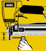
● This tool is equipped with a depth control safety element. To adjust the depth of the staple being driven, loosen the screw and slide the lower safety element up or down and lock in place by tightening the screw. Be sure the safety element moves freely after adjustment. A malfunctioning safety element can cause a fastener to be discharged accidentally.
