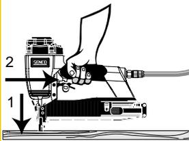
● With a "Dual-Action" trigger, nails can be driven two ways:
