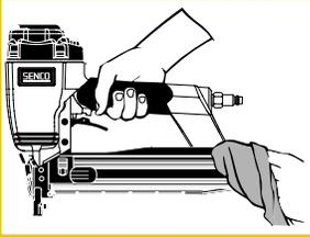
● Wipe tool clean daily and inspect for wear. Use non-flammable cleaning solutions only if necessary – DO NOT SOAK. **CAUTION:** Such solutions may damage O-rings and other tool parts.
