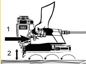
● With a "Restrictive" trigger, nails can only be driven one way. First depress safety element against work surface then pull trigger. This feature is helpful when precise fastener placement is required. Read the "Customer Satisfaction and Safety Reminder" (CSSR) in the tool and fastener boxes for safety information regarding the Dual Action and Restrictive triggers. Under certain conditions, the Restrictive trigger may reduce the possibility of injury to you or to others working with you.
