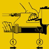
● Move the sides of the magazine up or down to adjust. Line up the holes in the sides of the magazine with the locating pins.
