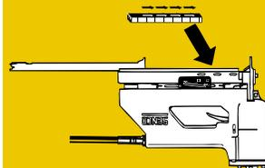
● Place strip of fasteners into magazine with printed side facing out and arrows pointed toward front of tool. Slide magazine rail closed.
