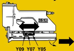
● To Load: Slide adjuster to correct fastener length. Pull latch and slide magazine rail to rear.
