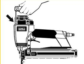
● All screws should be kept tight. Loose screws result in unsafe operation and parts breakage.
