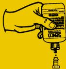
● Squirt Senco pneumatic oil (5 to 10 drops) into the air inlet twice daily. (Depending on frequency of tool use.)
