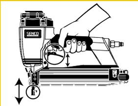
● With tool disconnected, make daily inspection to assure free movement of safety element and trigger. Do not use tool if safety element or trigger sticks or binds.
