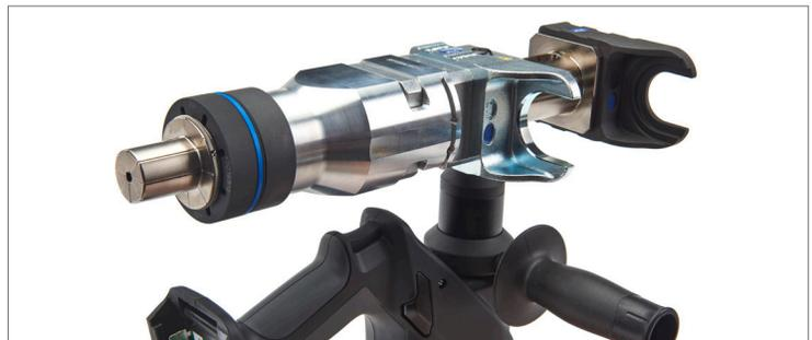
9. If necessary, swap and flip the compression jaws to make it easier to compress the fitting assembly.
