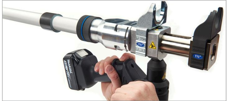
14. To compress EVERLOC+ sleeve, the black compression jaw must be placed on the fitting and the silver jaw must be placed behind the sleeve. It may be necessary to control the pipe during installation. Be sure to keep your hands and fingers clear of the moving parts.
