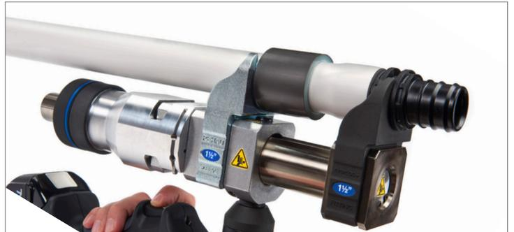
15. To release the hydraulic pressure and return the tool to its starting position, press the release button.
