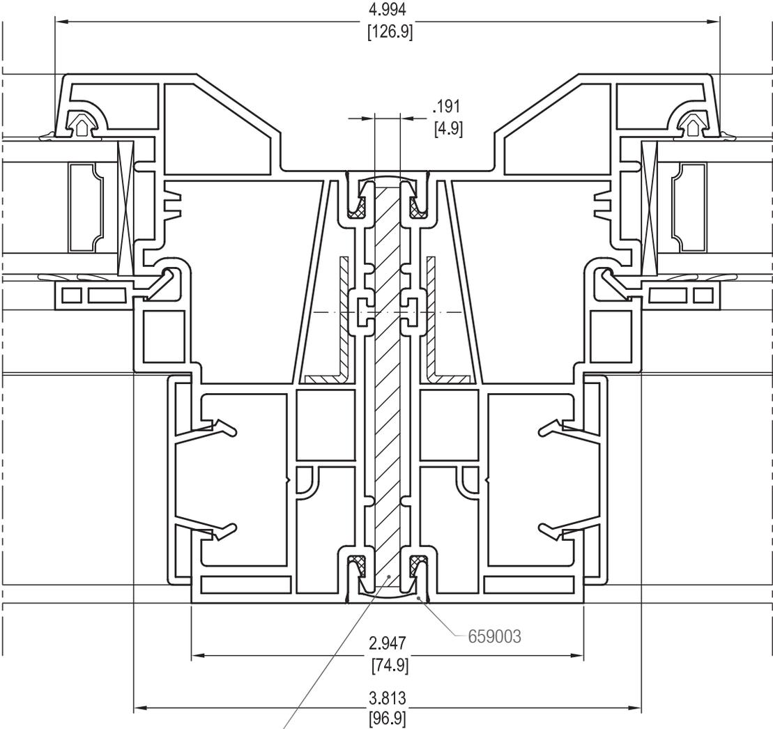
Structural reinforcement material as required, up to 3/16 in (4.8 mm) x 3 in (76 mm)
