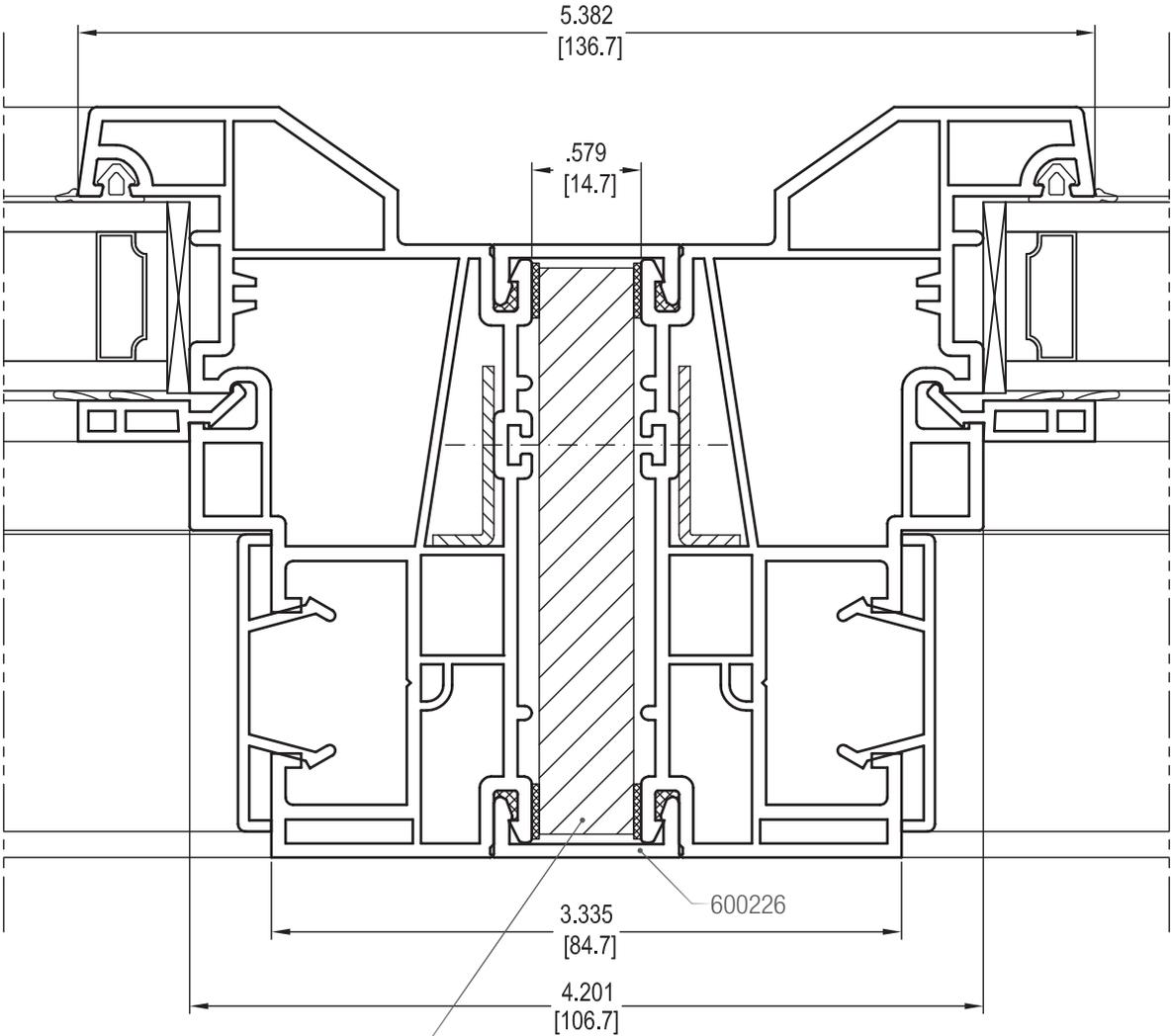
Structural reinforcement material as required, up to 1/2 in (12 mm) x 3 in (76 mm)
