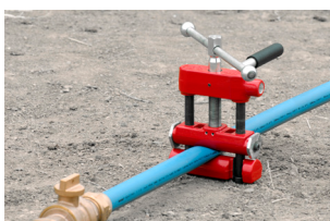
Fig. 12: Pipe in squeeze-off tool
