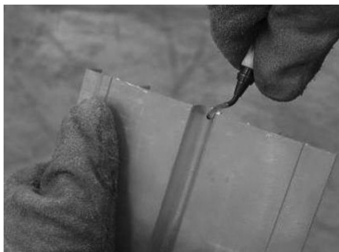
Fig. 16: Deburring sharp edges
