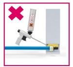
It is the responsibility of the installing contractor to verify compatibility of any chemicals that come into contact with the PPSU fittings. In addition, the installing contractor should ensure that other trades on the job site do not allow external chemicals to come into contact with the PPSU fittings. If it is required to protect the fittings, use only REHAU recommended protective tapes for wrapping of REHAU F1960 joints.
