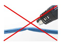
No approved repair method; kink must be cut and coupling installed
