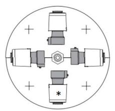
The red pull-out tab is provided to reduce the force of the actuator when installing on the manifold. The manifold valve remains open when the red tab is in place. Keep the red tab in place when installing the actuator on the manifold. Remove the red tab after installing the actuator.
