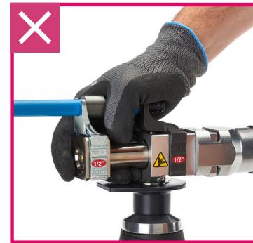
14. To release the hydraulic pressure and return the tool to its starting position, press the release button.
