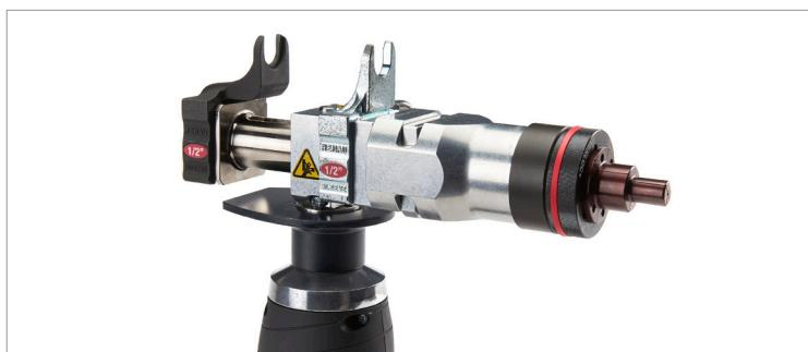
9. If necessary, remove the expansion adapter to make it easier to compress the fitting assembly. Press the release lever and slide the adapter off the expansion slot to remove.
