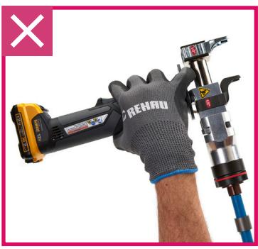
13. To compress EVERLOC+ sleeve, the black compression jaw must be placed on the fitting and the silver jaw must be placed behind the sleeve. It may be necessary to control the pipe during installation. Be sure to keep your hands and fingers clear of the moving parts.
