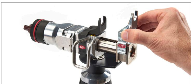
6. If necessary, the tool head can be rotated to make installation easier. The collar rotates with the tool head. Have a missing or damaged collar repaired or replaced before use.
