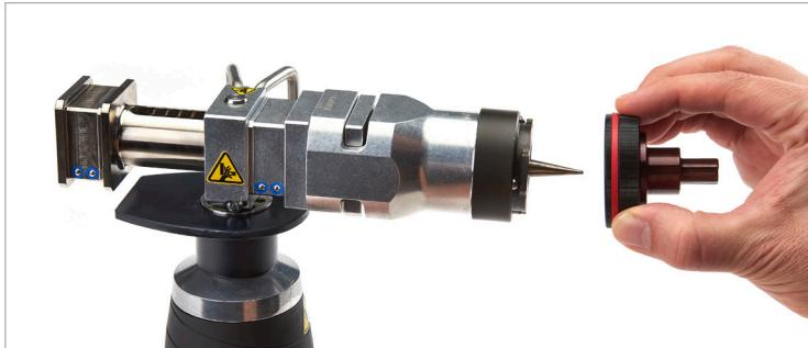
5. Slide the compression jaws into the compression slots.
